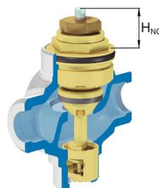
**Combination of valve and closing dimension adapter**
