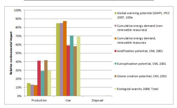
The relationship of the contributions made by the utilisation in comparison to those made by the reduction and disposal depends on the intensity of the utilisation (utilisation scenario).
