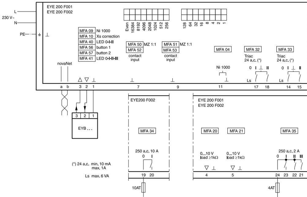
Connection diagram for EYE200F001 and EYE200F002 – “fan coil unit system – 4-pipe”
