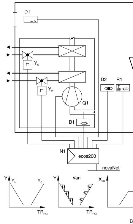
Fan coil temperature controller with 4-pipe system Heating with radiator
