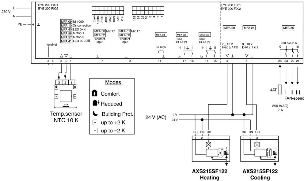
Connection diagram for EYE200F001 and EYE200F002 – “chilled-ceiling system”
