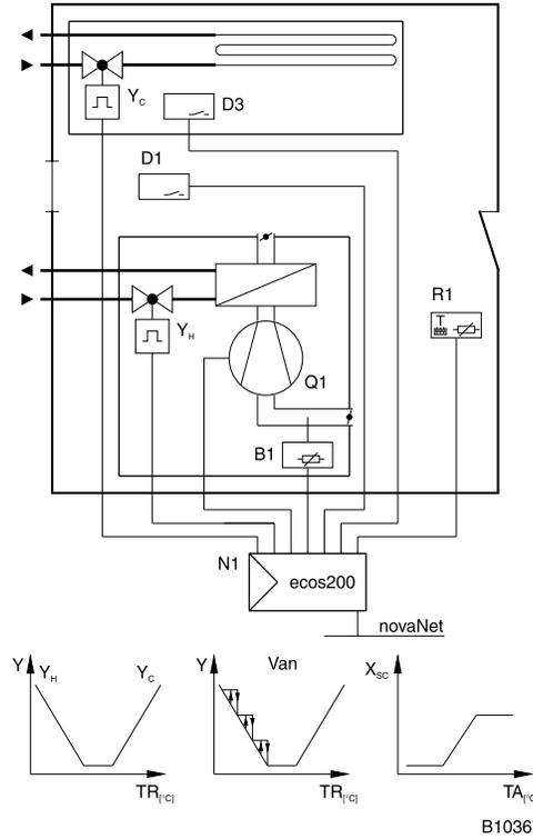
Fan coil temperature controller with 2-pipe system
