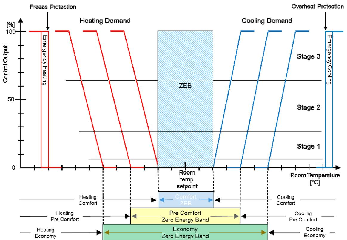
Fig. 1: Setpoint pairs for different energy levels
