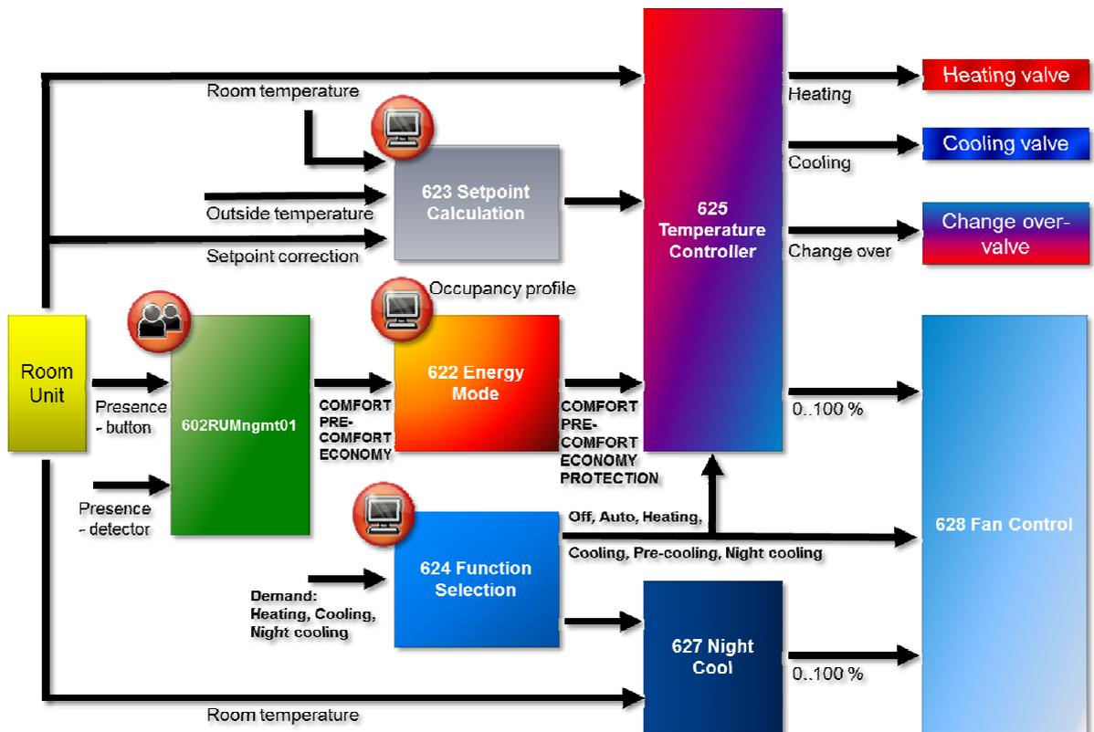
Fig. 2: Climate package block diagram from SAUTER
