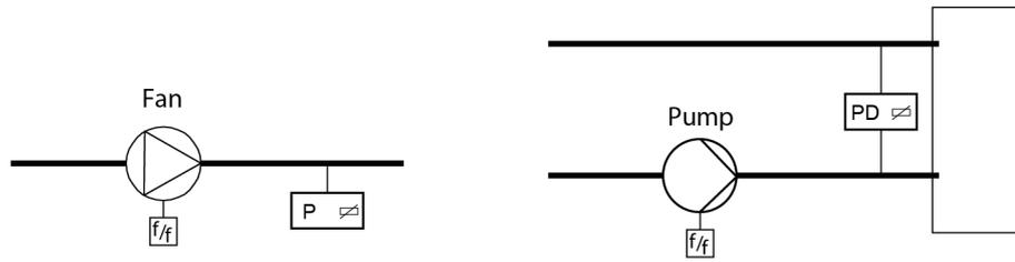
The output signal will increase when the pressure signal falls below the setpoint value.
