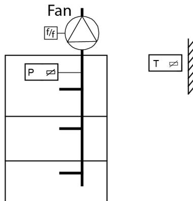
The output signal will increase when the pressure signal falls below the setpoint value.
