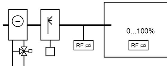
The control mode consists of a general control in sequence. A neutral zone can be set between AO1 and AO2.
