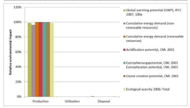
The relationship of the contributions made by the utilisation in comparison to those made by the reduction and disposal depends on the intensity of the utilisation (utilisation scenario).
