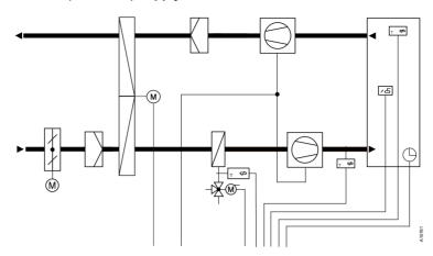
A P-PI cascade controller is used. Maximum and minimum limits can be set for the supply air. A return-air or room-temperature sensor must be used.
