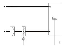
A PI control loop is used. A min/max limit for the output is possible.
