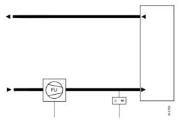
A PI control loop is used. The pressure transmitter must have an output signal of 0...10 V. The measuring range can be set to up to 2500 kPa.
