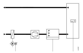
A PI-controller is used. With humidity control, AO1 is used to humidify (positive control) and AO2 is used to dehumidify (negative control).
