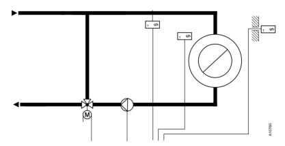
A PI control loop is used. The setpoint for the supply temperature is defined automatically depending on the outside temperature.
