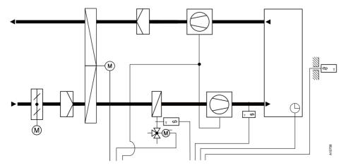
A PI control loop is used. The setpoint is defined automatically depending on the outside temperature.
