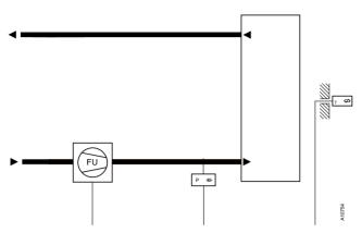
A PI control loop is used. The pressure setpoint is defined based on the outside temperature, and the temperature range is set to 20...60 °C. The pressure transmitter must have an output signal of 0... 10 V. The measuring range can be set to up to 2500 kPa.
